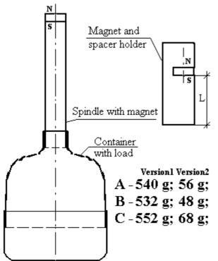
Measurement of the force of attraction and repulsion of magnets-tablets using an electronic scale - variability of weight indications - every 2 grams. A - weight of the container with the load,
